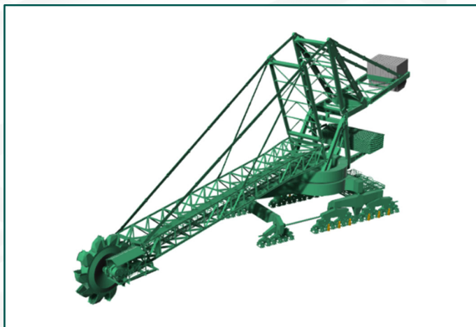
Figure 11: Example showing detailed 3D modelling of a bucketwheel reclaimer, which was created using the 3D modelling software Rhinoceros.
